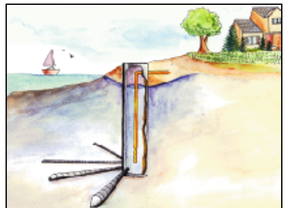
Diagram of Riverbank Infiltration System
